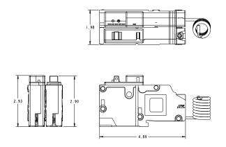
Figure 3. Two-pole smart breaker
