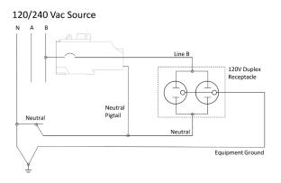
Figure 6. Two-pole 240V load application sourced by 120/240 Vac
